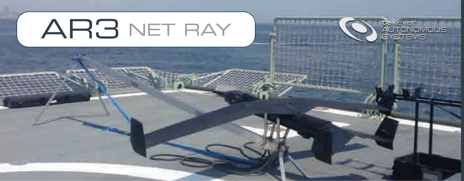
The **AR3 NET RAY** is a fully autonomous small UAS designed to support multiple missions, including Intelligence, Surveillance, Target Acquisition and Reconnaissance (ISTAR) and Communications Relay missions.
